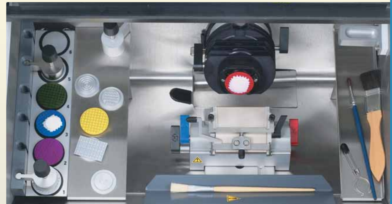
SPACIOUS CRYOCHAMBER AND COLOR-CODED CRYOCASSETTES: Facilitates easy patient / specimen identification.
