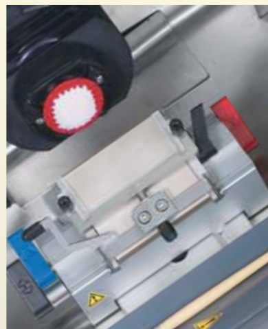
NEW BLADE HOLDER: Lateral movement of blade holder eliminates need to unclamp and re-clamp blade. Maximizes blade usage. Color coded levers identify lever functions.
