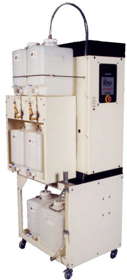
40-Liter Cart-mounted Recycler* 78 cm wide, 170 cm high, 77 cm deep
